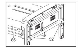
Raise the Uprights (85) to the vertical position. Remove the three #8 x 3/4" Screws (7) from the Hood (33), and carefully pivot the Hood off.
